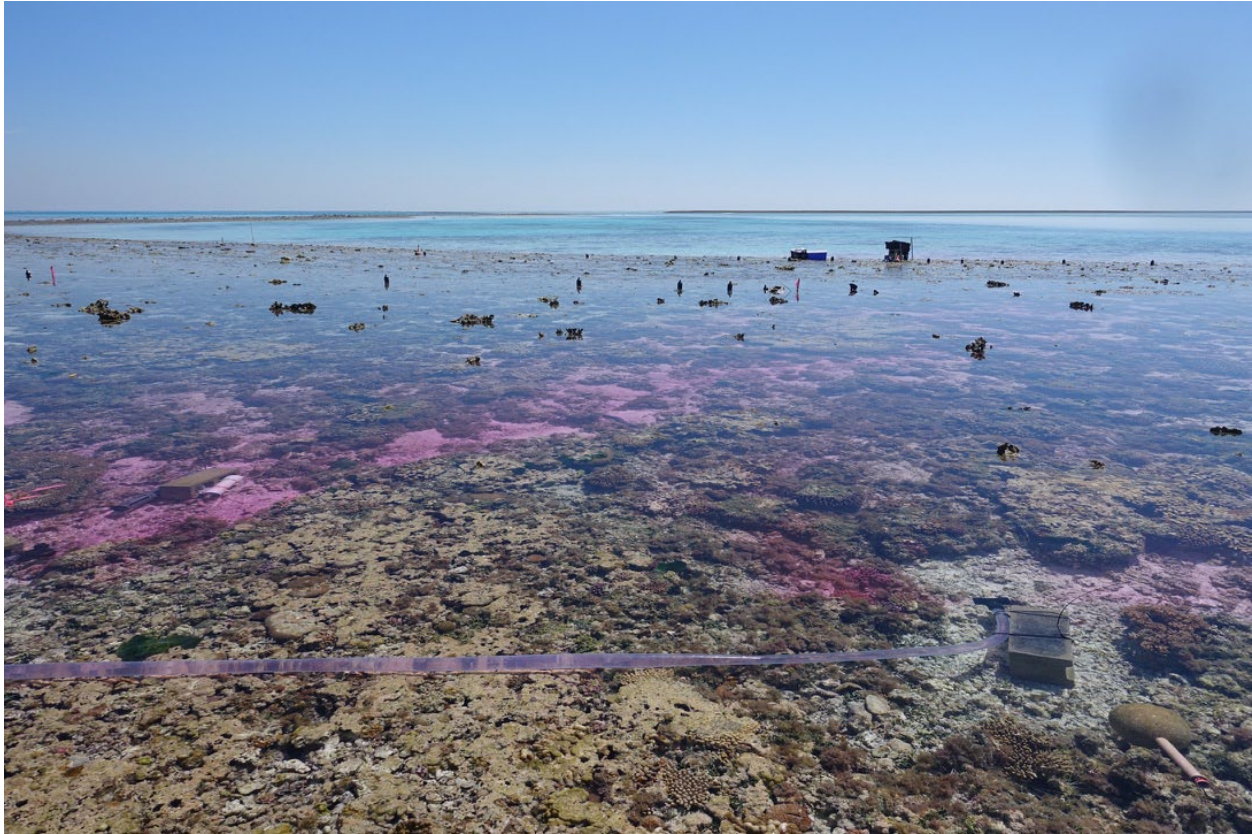
356 357 Figure 1. Rhodamine dye flowing over a coral reef flat study site during a study in One Tree 358 Island, Australia (Albright et al. 2016). NaOH was used as an active tracer to raise alkalinity, and 359 rhodamine was used as a passive tracer to account for mixing and dilution. Changes in the 360 alkalinity-dye ratios were used to isolate the change in alkalinity flux that was associated with an 361 increase in net community calcification on the reef flat.
