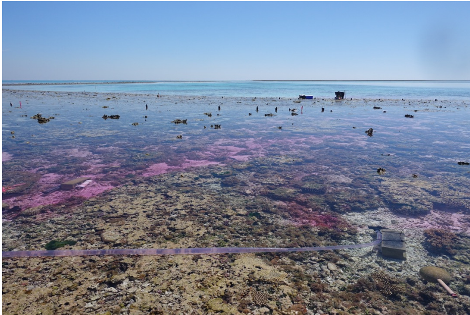
404 405 Figure 1. Rhodamine dye flowing over a coral reef flat study site during a study in One Tree 406 Island, Australia (Albright et al. 2016). NaOH was used as an active tracer to raise alkalinity, and 407 rhodamine was used as a passive tracer to account for mixing and dilution. Changes in the 408 alkalinity-dye ratios were used to isolate the change in alkalinity flux that was associated with an 409 increase in net community calcification on the reef flat.
