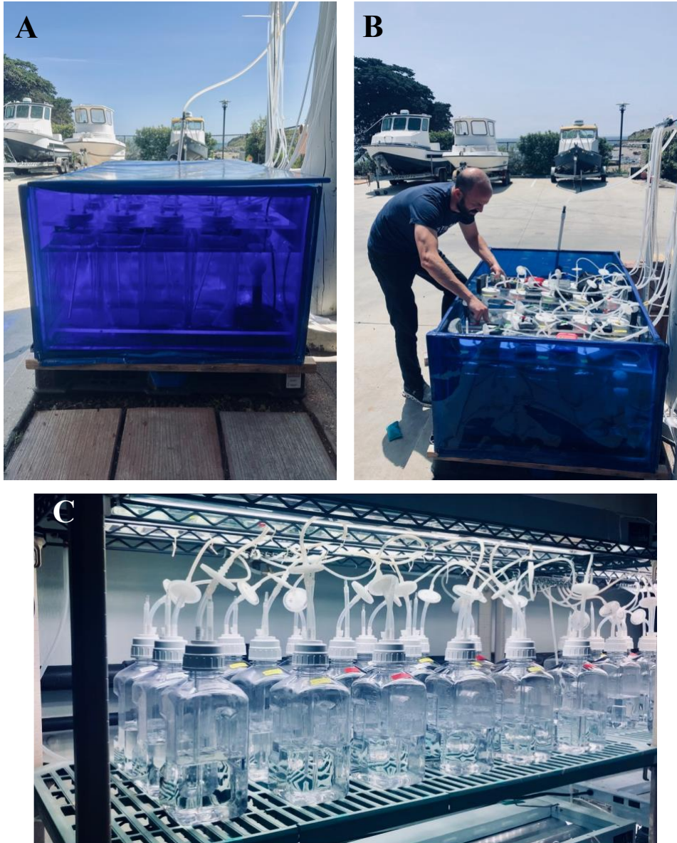
595 596 597 Figure 2. A, B: Portable incubator with blue filters to adjust photosynthetically active radiation (PAR). A scalar 598 PAR sensor (LI-COR) can be observed within the incubator (A, right side). C: laboratory experiment using aeration 599 and sacrificial replication. Images were taken by James Gately (A, C) and Sylvia Kim (B).
