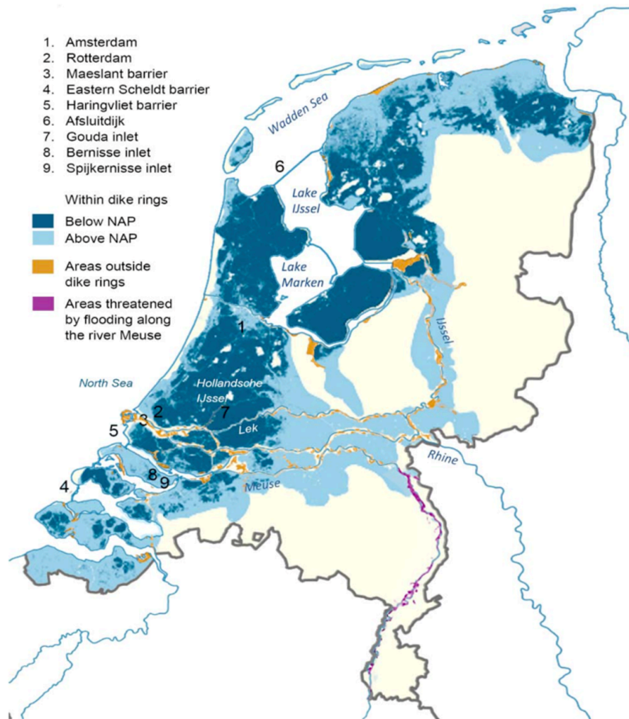
Figure 5: Map of the Netherlands showing flood prone zones (blue shadings) and features of the water management system. NAP is the Amsterdam Ordnance Level which is the reference plane for sea level height in the Netherlands. Extracted from Haasnoot et al., 2020.
