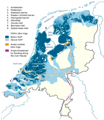
Figure 1. Map of the Netherlands showing flood prone zones (blue shadings) and features of the water management system (adapted from PBL [58]). N.A.P. is the Amsterdam Ordnance Level which is the reference plane for sea level height in the Netherlands.
