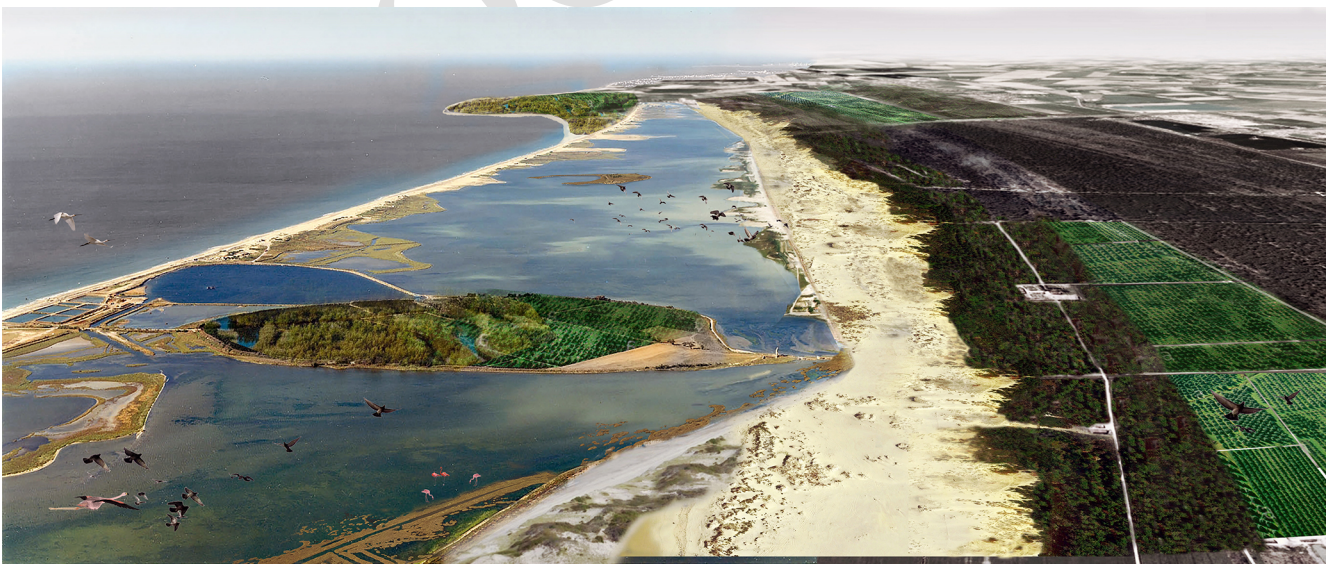
Figure 4. Computer-generated image of possible configuration in 2100 (considering the IPCC RCP8.5 projections for SLR) in the southern coastal area of the municipality of Ravenna (Lido di Classe–Lido di Dante), according to a dynamic and evolutive approach, considering managed realignment of the coastline, the construction of a new dune line and the partial environmental transformation of the territory. The original source of this figure is Lobosco and Mencarini (2023).
