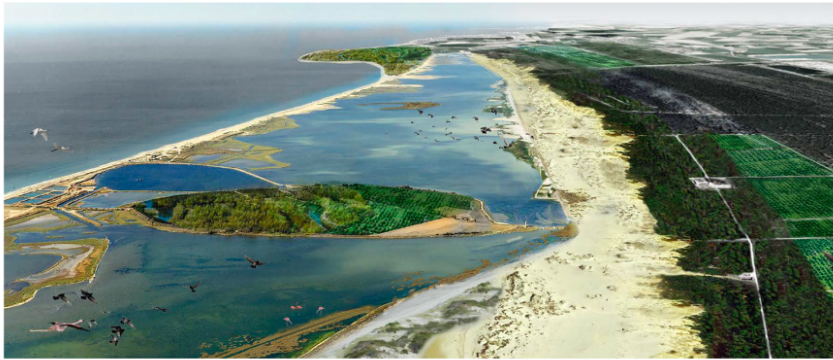
Fig. box.2: computer-generated images of possible configuration at 2100 (considering the IPCC RCP8.5 projections for SLR) in the southern coastal area of the Ravenna Municipality (Lido di Classe-Lido di Dante), according to: a) a rigid-conservative approach, with maintenance of the coastal defense structures and the coastline position, with a prevalent agricultural destination in internal areas; b) a dynamic and evolutive approach, considering managed realignment of the coastline, the construction of a new dune line and the partial environmental transformation of the territory.
