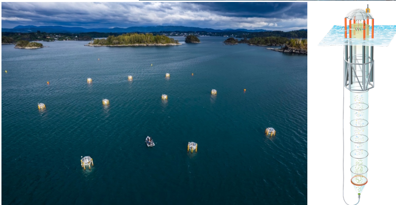
601 Figure 1. Pelagic mesocosm facilities currently used in OAE research. top left : Land-based mesocosms (1 m 3 ) 602 at the University of Vigo, Spain. top right : In situ on-shore mesocosms (10 m 3 ) operated by GEOMAR, here 603 employed on Gran Canaria, Spain. bottom left : Kiel Off-Shore Mesocosms for Ocean Simulations (KOSMOS), 604 here employed in the Raunefjord, Norway. bottom right : Sketch of a KOSMOS mesocosm unit (55 m 3 ). 605 Photo/graphic sources: ul : Daniela Basso, University of Milano-Bicocca, ur : Ulf Riebesell, GEOMAR, bl : Uli 606 Kunz, br : Rita Erven, GEOMAR.
