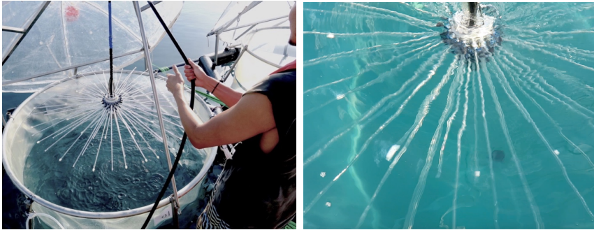
Figure 5: Left : Distribution device used for alkalinity addition; by moving it up and down in the water column during alkalinity injection at constant speed a uniform alkalinity enhancement can be achieved. Right : Milky water at the outlet of the injection tubes indicates temporary precipitation which, however, quickly disappears as the highly concentrated alkalinity solution dilutes. Photo sources: Ulf Riebesell
