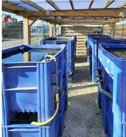
617 Figure 3: In the benthic mesocosms at the University of Antwerp the dissolution kinetics of silicate minerals and 618 the impacts on the benthic fauna in coastal environments are monitored since 2019. The system comprises 20 619 units with two stacked tanks, the upper tank is housing the benthic ecosystem, and the lower tank is functioning 620 as a water reservoir. Natural sediment of 40 sediment height with a mean grain size of 123 \mu\text{m} (3.0 phi) was 621 collected from an intertidal sand flat in the Oosterschelde (Netherlands) and mixed with olivine sand of similar 622 grain size. Water from the Easter Scheldt Estuary (salinity 32-35) is used to conduct flux-sessions of 5 weeks 623 (weekly sampling). At the end of each session, the total volume of water in each unit (~500 L) is renewed 624 (Drawing: A. Hylén, Photo: M. Kreuzburg https://www.coastal-carbon.eu/ , Geobiology, University of Antwerp).
