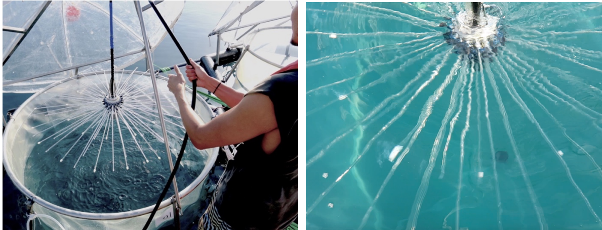
642 Figure 5: Left : Distribution device used for alkalinity addition; by moving it up and down in the water column 643 during alkalinity injection at constant speed a uniform alkalinity enhancement can be achieved. Right : Milky water 644 at the outlet of the injection tubes indicates temporary precipitation which, however, quickly disappears as the 645 highly concentrated alkalinity solution dilutes. Photo sources: Ulf Riebesell
