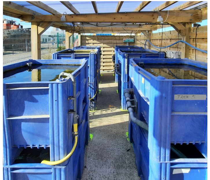
616 Figure 3: In the benthic mesocosms at the University of Antwerp the dissolution kinetics of silicate minerals and 617 the impacts on the benthic fauna in coastal environments are monitored since 2019. The system comprises 20 618 units with two stacked tanks, the upper tank is housing the benthic ecosystem, and the lower tank is functioning 619 as a water reservoir. Natural sediment of 40 sediment height with a mean grain size of 123 \mu\text{m} (3.0 phi) was 620 collected from an intertidal sand flat in the Oosterschelde (Netherlands) and mixed with olivine sand of similar 621 grain size. Water from the Easter Scheldt Estuary (salinity 32-35) is used to conduct flux-sessions of 5 weeks 622 (weekly sampling). At the end of each session, the total volume of water in each unit (~500 L) is renewed 623 (Drawing: A. Hylén, Photo: M. Kreuzburg https://www.coastal-carbon.eu/ , Geobiology, University of Antwerp).
