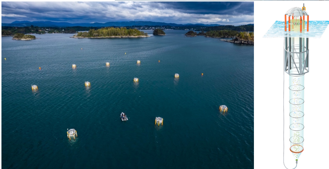
596 Figure 1. Pelagic mesocosm facilities currently used in OAE research. top left : Land-based mesocosms (1 m 3 ) 597 at the University of Vigo, Spain. top right : In situ on-shore mesocosms (10 m 3 ) operated by GEOMAR, here 598 employed on Gran Canaria, Spain. bottom left : Kiel Off-Shore Mesocosms for Ocean Simulations (KOSMOS), 599 here employed in the Raunefjord, Norway. bottom right : Sketch of a KOSMOS mesocosm unit (55 m 3 ). 600 Photo/graphic sources: ul : Daniela Basso, University of Milano-Bicocca, ur : Ulf Riebesell, GEOMAR, bl : Uli 601 Kunz, br : Rita Erven, GEOMAR.
