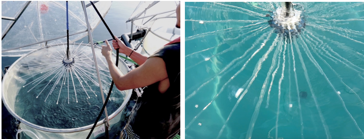
638 Figure 5: Left : Distribution device used for alkalinity addition; by moving it up and down in the water column 639 during alkalinity injection at constant speed a uniform alkalinity enhancement can be achieved. Right : Milky water 640 at the outlet of the injection tubes indicates temporary precipitation which, however, quickly disappears as the 641 highly concentrated alkalinity solution dilutes. Photo sources: Ulf Riebesell
