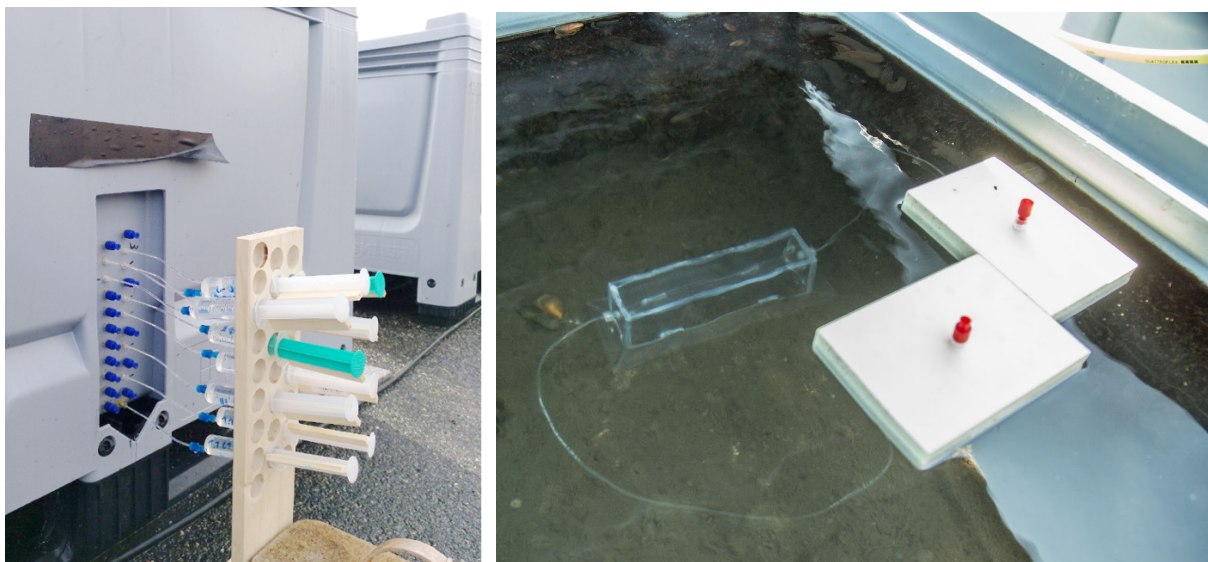
654 Figure 6. left : Pore fluid sampling using rhizons. right : benthic incubation chamber to assess alkalinity 655 enhancement with respect to mineral dissolution in benthic mesocosm experiments. Photo sources: left Sonja 656 Geilert, right Michael Fuhr, GEOMAR.
